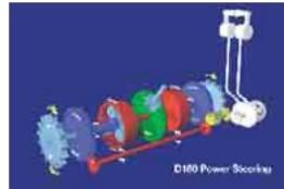
A hydraulic motor increases the speed of one track and decreases the speed of the opposite one to generate power steering.
