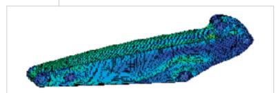
Booms and Arms have been redesigned using advanced CAD (Computer Aided Design) and FEM (Finite Elements Methodology) Systems to get higher strength **only** in those areas where stresses are concentrated.
