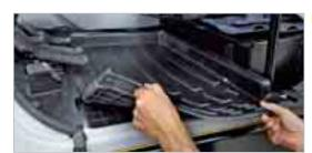
Detachable two-piece floormat with handles for easy removal. A floor drain is located under the mat to facilitate inside cab cleaning.
