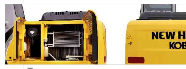
he simplified layout of all vital components of the New Holland E195B under both the right and the left side panels makes maintenance much easier, less time consuming and less costly, and provides much better access for servicing. There is plenty of room in all compartments and most components are positioned in such a way to enable easy access from ground level. **An elegant and modern design added to state-of-the-art technology.**
