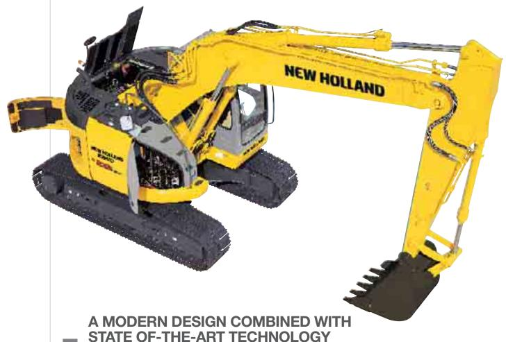
he simplified layout of the New Holland E225BSR & E235BSR components, positioned under both the right and the left side panels, enables easy access from ground level and makes maintenance and inspections quicker and less expensive. Reduced maintenance and service costs to keep machines in perfect condition: low maintenance costs, high reliability and durability, minimised owning and operating costs for your improved profit.
