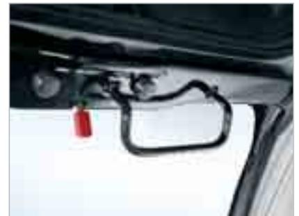
One-touch lock release simplifies opening and closing the front window, while a new mechanism makes it lighter.
