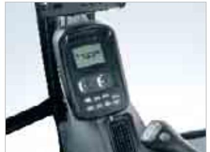
The newly designed **A.E.P. Information Display** features analogical gauges which provide one sight advice, regardless of the operating environment. The digital display screen has been enlarged to further enhance visibility. Maintenance information is clearly displayed and the self-diagnostic function provides an early warning detection of malfunctions. Details of any previous breakdown or malfunction are also stored.
