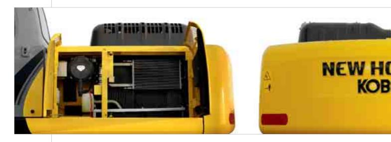
he simplified layout of all vital components of the New Holland E265B under both the right and the left side panels makes maintenance much easier, less time consuming and less costly, and provides much better access for servicing. There is plenty of room in all compartments and most components are positioned in such a way to enable easy access from ground level. **An elegant and modern design added to state-of-the-art technology.**
