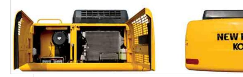
he simplified layout of all vital components of the New Holland E485B under both the right and the left side panels makes maintenance much easier, less time consuming and less costly, and provides much better access for servicing. There is plenty of room in all compartments and most components are positioned in such a way to enable easy access from ground level. **An elegant and modern design added to state-of-the-art technology.**
