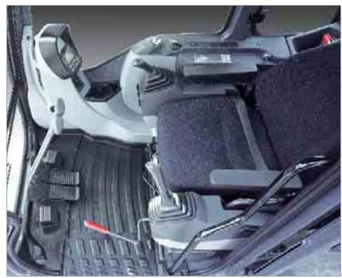
materials create an elegant feeling. Rigid cab construction, combined with six silicon liquid filled viscous dampers, minimises vibrations.
