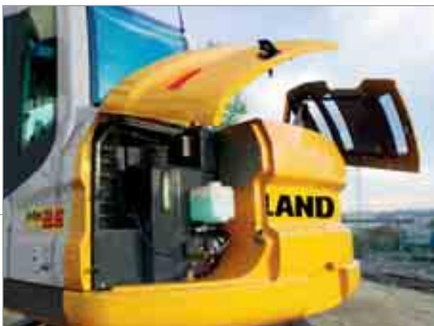
**D**iesel tank with level indicator.
