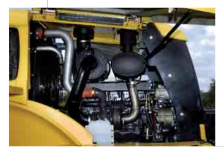
An **Automatic power mode** can be also selected to automatically match the engine power curve, between maximum power and standard power, to the machine application.
