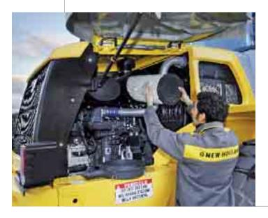
he W130B is designed for simple and easy maintenance and service procedures thanks to its excellent ground level access to all the most important components and to the new high-tech digital display located on the dashboard, which keeps the operator fully aware of all machine main functions, such as engine and transmission diagnostics, error reporting and warning prompts.
