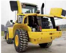
hey give immediate access to most of the engine components, including the high pressure injection pump, alternator, fuel/water separator, engine oil filter, fuel filter, air filter and the engine electronic control panel. Access to the hydraulic tank is provided by a third liftable panel, located on the top of the engine hood, behind the cab.
