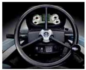
he W170B is designed for simple and easy maintenance and service procedures thanks to its excellent ground level access to all the most important components and to the new high-tech digital display located on the dashboard, which keeps the operator fully aware of all machine main functions, such as engine and transmission diagnostics, error reporting and warning prompts.
