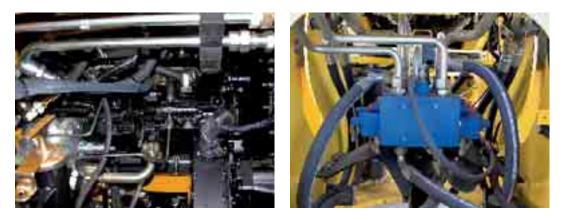
he **closed centre** pilot control valve allows simultaneous under every load and engine speed condition: an outstanding feature so far offered only by best in market hydraulic excavators. Controls are power assisted, with electromagnetic detent and the loader section of the control valve includes floating function.
