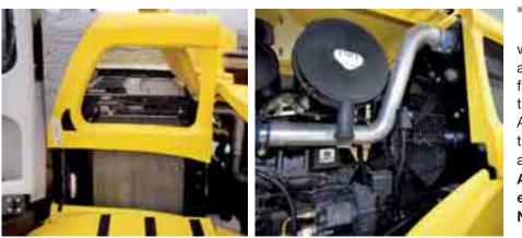
he variable speed hydrostatic fan, with eight plastic blades, is automatically actuated by a thermostatic sensor, drawing fresh and clean air from outside through the radiators and the hydraulic oil tank. A switch in the cab allows the operator to select the fan counter rotation for easy and automatic radiator cleaning. A really comfortable, durable and efficient innovation offered by New Holland.
