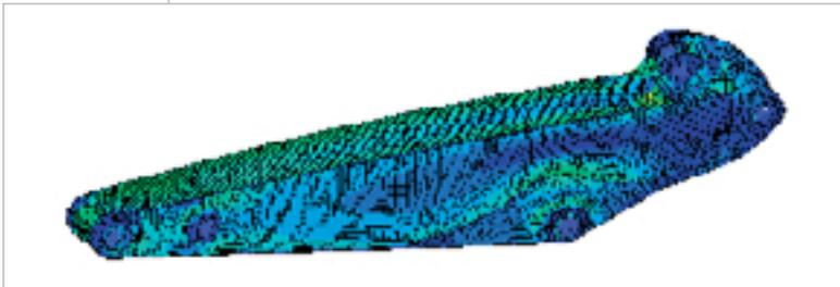
**B**ooms and Arms have been redesigned using advanced CAD (Computer Aided Design) and FEM (Finite Elements Methodology) Systems to get higher strength **only** in those areas where stresses are concentrated.
