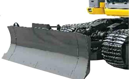
The E150 Blade Runner's blade has a bolt-on reversible cutting edge
