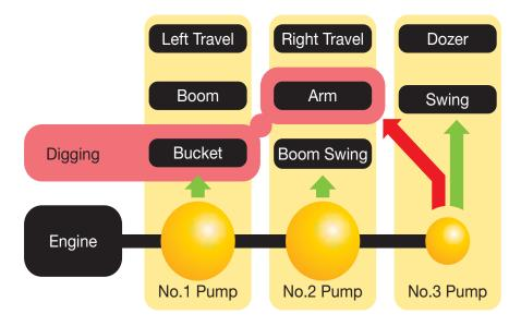
The instant the machine begins to dig, extra output from the third pump (which otherwise powers the swing and dozer circuits) is directed to the arm circuit for added power. This ensures fast and smooth arm operation even under heavy loads.
