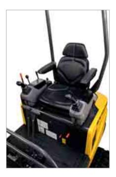
A user-friendly operating environment designed for long days of productive work and minimal operator fatigue: hand or foot operated travel controls, readily visible instrument panel, unrestricted visibility in all directions.
