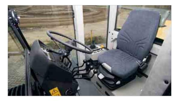
Besides high operating comfort and visibility, the oversized ROPS/FOPS cab also offers the necessary safety and a seat that gives the driver a firm hold even when working along slopes. Sliding doors permit easy access from both sides. Moreover, the cab is mounted on the rear frame: a highly valuable advantage versus main competitors and in terms of operators comfort and convenience:
