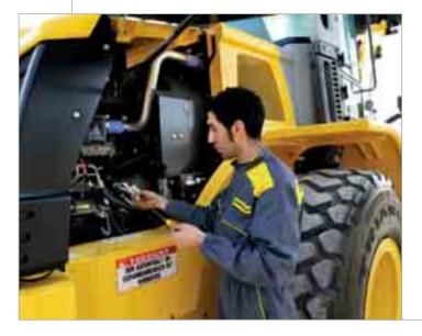
he W110B is designed for simple and easy maintenance and service procedures thanks to its excellent ground level access to all the most important components and to the new high-tech digital display located on the dashboard, which keeps the operator fully aware of all machine's main functions, such as engine and transmission diagnostics, error reporting and warning prompts.
