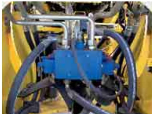
The **closed centre** pilot control valve allows simultaneous under every load and engine speed condition: an outstanding feature so far offered only by best in market hydraulic excavators. Controls are power assisted, with electromagnetic detent and the loader section of the control valve includes floating function. Hydraulic and Steering: an integrated system which features operator comfort as well as top class safety, controllability and efficiency.
