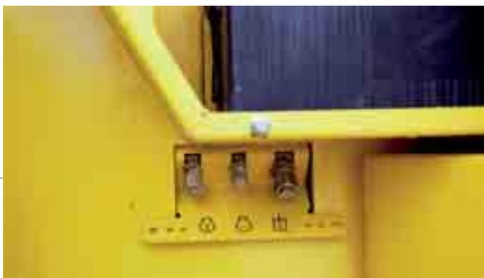
**G**rouped together in a protected and easily-accessible remote position on the rear left side of the machine are the engine oil, coolant and hydraulic oil valves, allowing easy and ecological discharge of fluids. All this adds up to maximum comfort, safety, efficiency and economy in the day-to-day use of the New Holland W170B.
