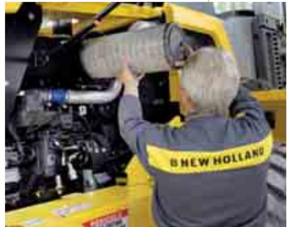
**T**hey give immediate access to most of the engine components, including the high pressure injection pump, alternator, fuel/water separator, engine oil filter, fuel filter, air filter and the engine electronic control panel. Access to the hydraulic tank is provided by a third liftable panel, located on the top of the engine hood, behind the cab.
