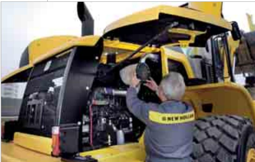
The W190B is designed for simple and easy maintenance and service procedures thanks to its excellent ground level access to all the most important components and to the new high-tech digital display located on the dashboard, which keeps the operator fully aware of all machine main functions, such as engine and transmission diagnostics, error reporting and warning prompts.
